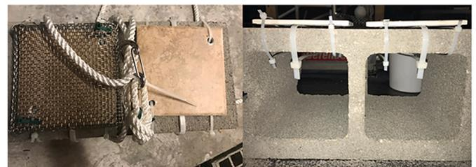
**Fig. 2.** Spat settlement collector comprising concrete cinderblock, ceramic settlement plates, 4 mm mesh stainless steel exclusion cage, and spacer for elevating settlement plates to form restricted spaces. Exclusion cages were used in 2018, but not in 2019.
